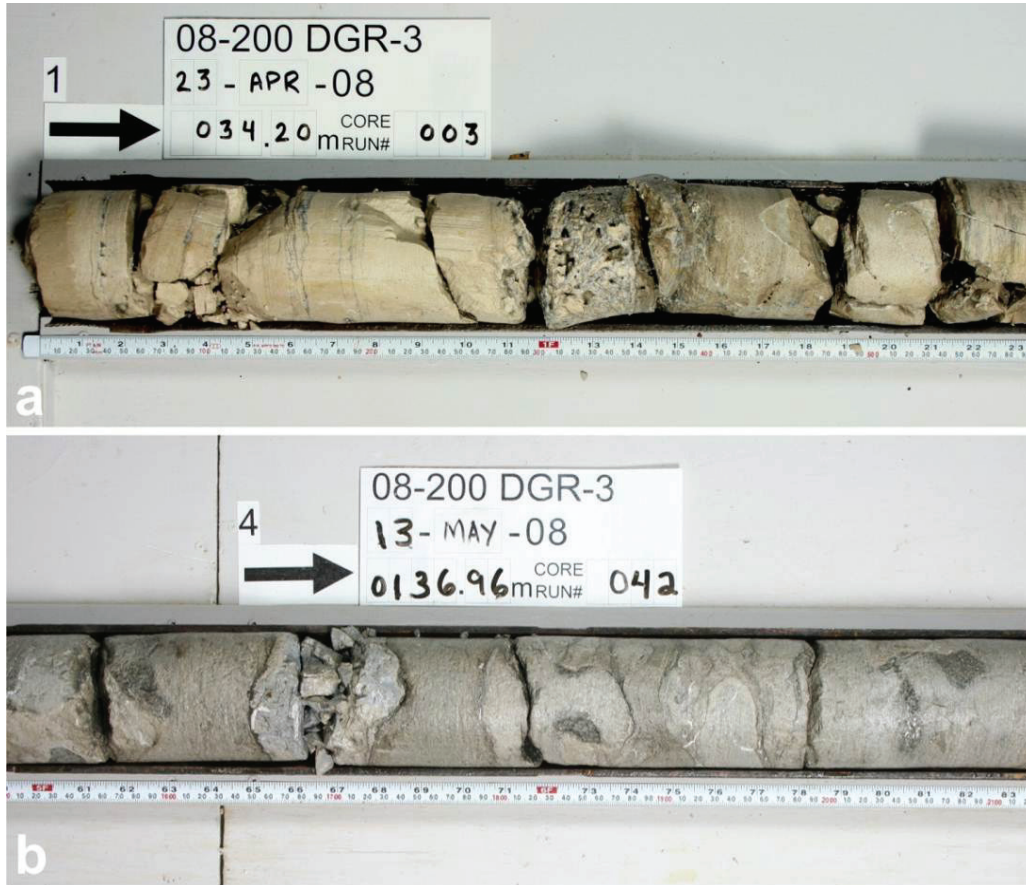
Figure 2.16: A) Core Photo from Shallow Devonian Lucas Formation Carbonates, Showing Karst Features and B) Remnant Paleokarst Horizon near the Top of the Bass Islands Formation
